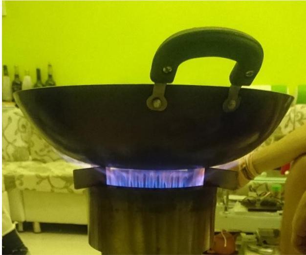
No improvements could be made with respect to the Belonio burner. Belonio placed burner holes along the periphery of the burner. The number of holes, the diameter of holes, the spacing of the holes, and the staggering of the two rings of holes – all remained the same. When any of these dimensions are changed, the burner does not function properly.
